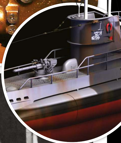
Above: U-48 had a secondary armament of an 88mm SK C/35 deck gun
